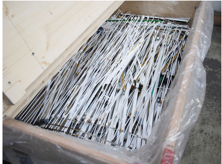
Figure 50. Safe storage in a box (with cover) for undamaged fluorescent tube [2].
