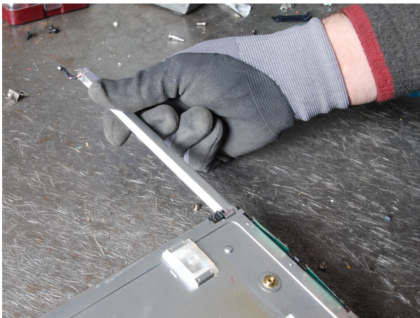
Figure 49. CCFL in a computer LCD screen [2].
