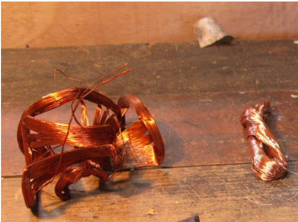
Figure 29. Recovered copper from a CRT monitor [2].
