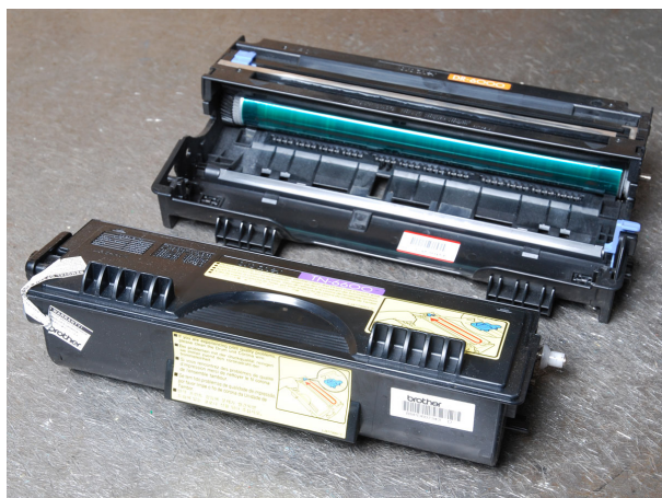
Figure 52. Toner Cartridge with photoconductive drum (green) [2].
