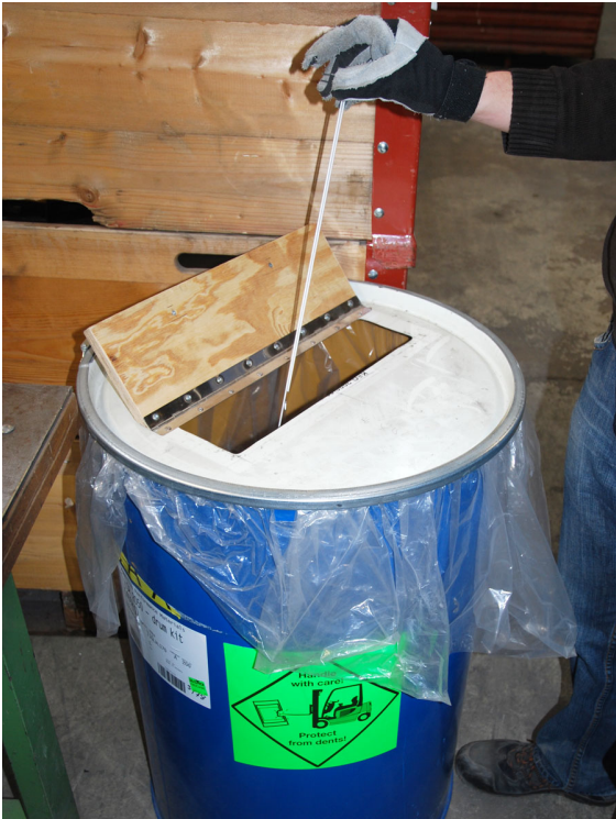
Figure 51. Barrel with a special cover to store broken fluorescent tubes in a safe way [2].
