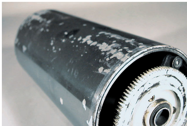
Figure 55. Selen-containing photoconductive drum [5].
