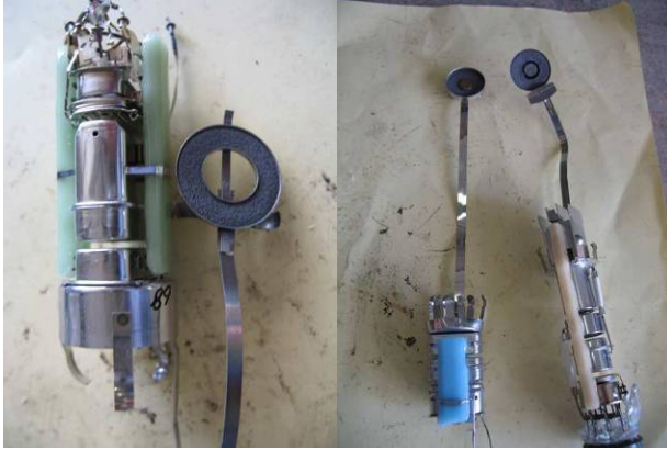
Figure 22. Electron gun & getter platelet [2].
